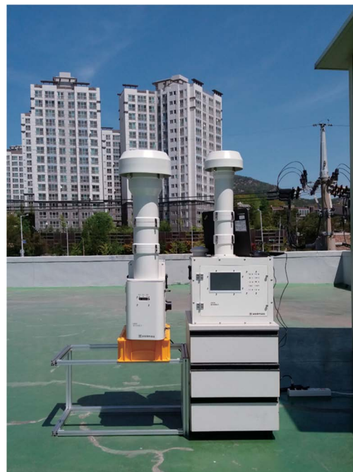
Fig. 2. BDS was installed on the top of the building to monitor and collect bio-aerosols in real-time: the detector (right) and the collector (left).
