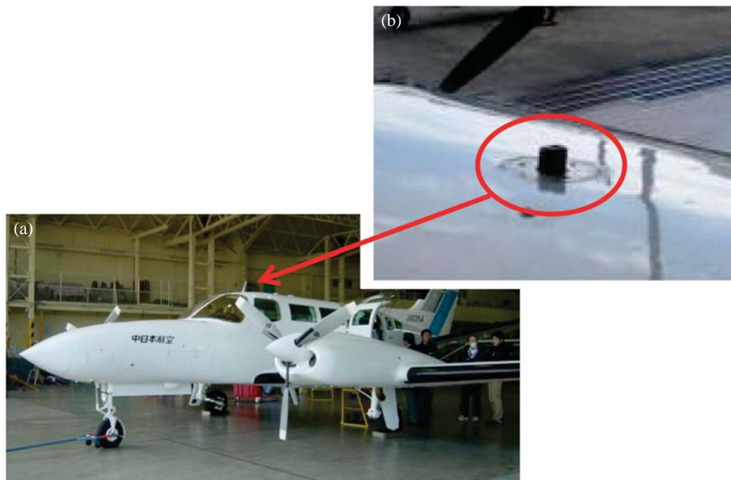
Fig. 1. Cessna 404 aircraft used for the direct sampling of atmospheric bioaerosol (a) and the outside of the inlet (b). The inlet was sterilized just before sampling.
